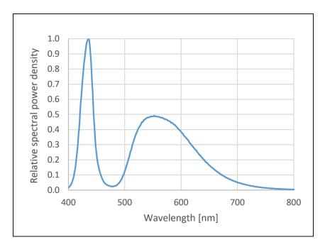
Figure 3. Typical white LED spectrum with blue pump and single YAG phosphor.
