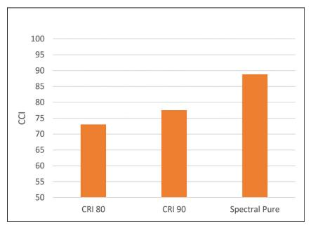
Figure 9. CCI results for typical camera flash LEDs and Spectral Pure.
