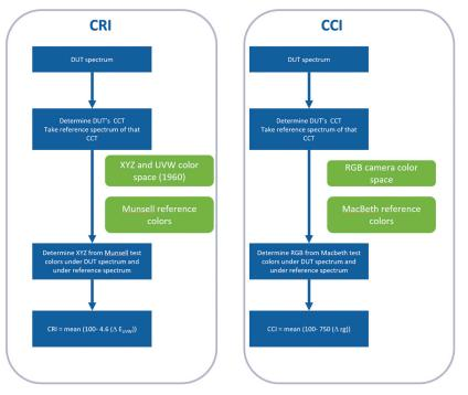
Figure 8. CRI vs. CCI procedure.
