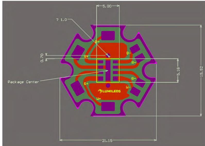
Figure 3b. Overall dimensions of example PCB footprint design for LUXEON 5052 RGBW. Dimensions in mm.
