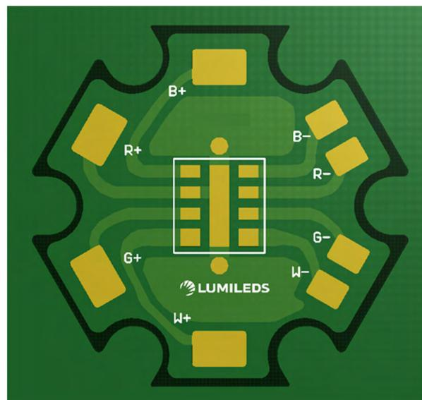
Figure 3a. Example PCB footprint design for LUXEON 5052 RGBW.
