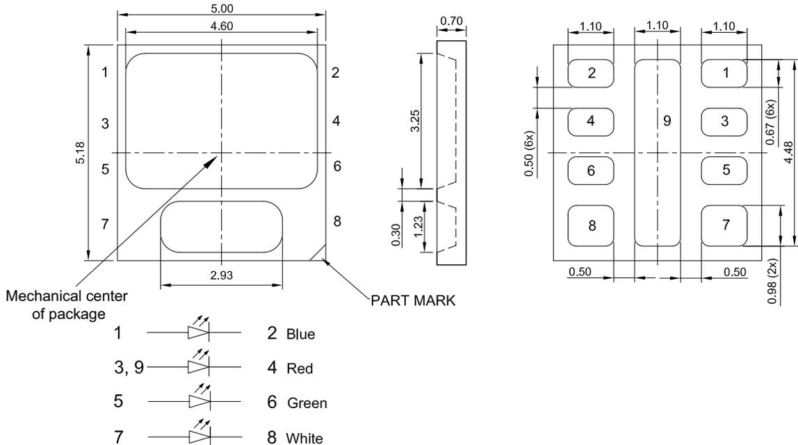
Figure 1. Mechanical Drawing of LUXEON 5052 RGBW.
