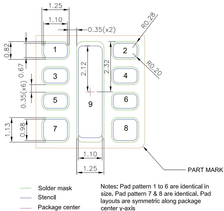
Figure 3c. Recommended PCB solder pad layout for LUXEON 5052 RGBW.
