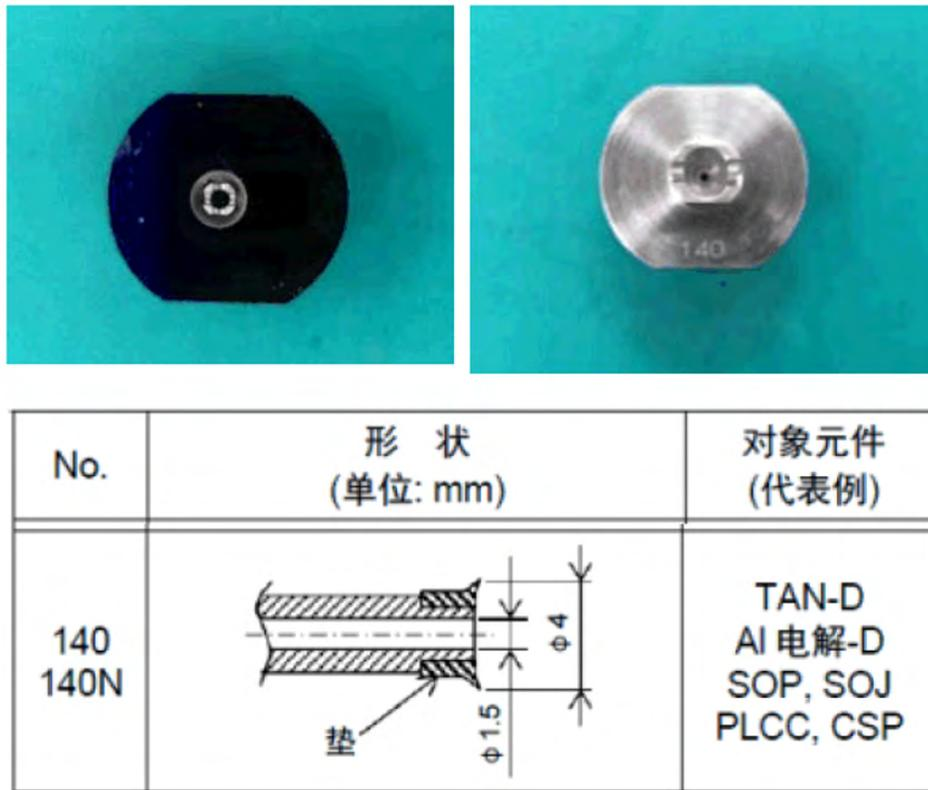
Figure 4. Example of tested nozzle: Panasonic 140 Nozzle.
