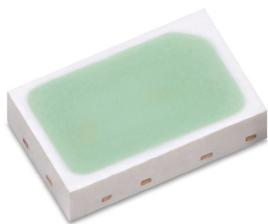
The LUXEON IR ONYX emitter features a continuous broadband infrared (IR) emission from 650 to 1100nm with superior light output characteristics. The product comes in an industry standard 2720 package and footprint for easy integration in existing designs. The LUXEON IR ONYX allows for new possibilities for miniaturization of spectroscopy and hyperspectral imaging applications in hand-held devices for mobile, industrial, and medical applications.
