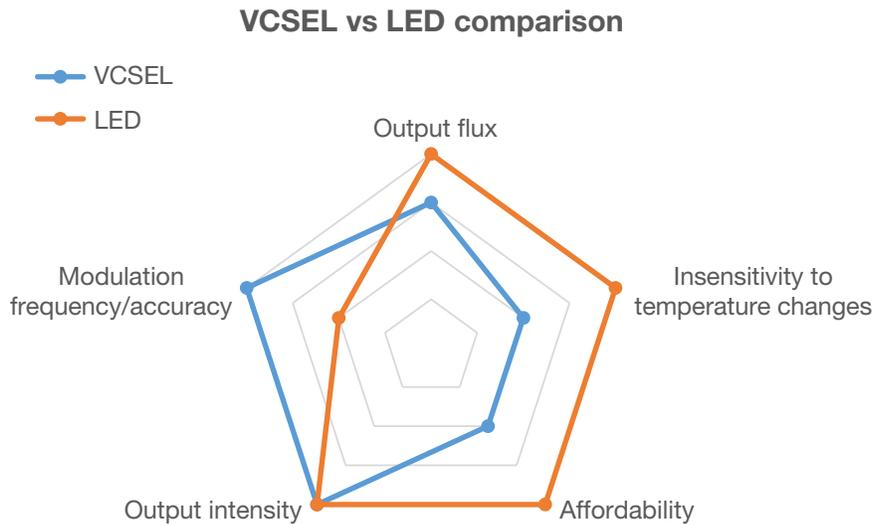
Figure 17. Qualitative comparison of IR VCSELs versus LEDs
