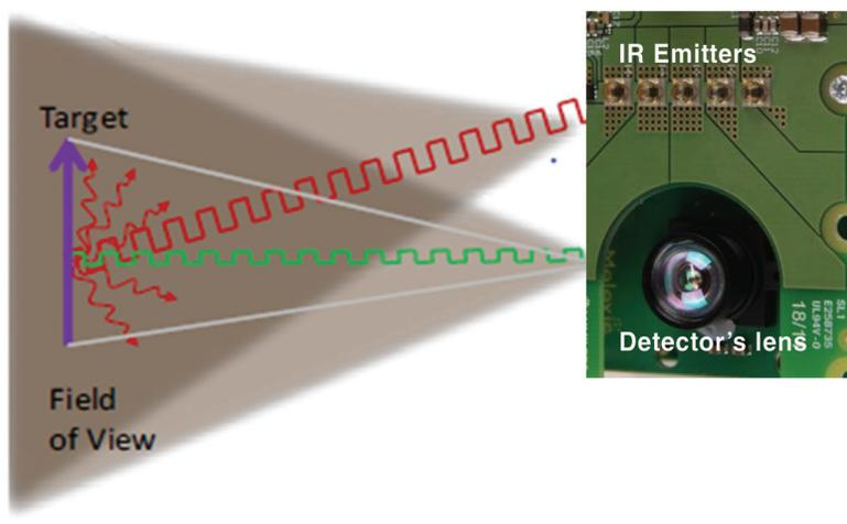
**Figure 1. Schematics of a TOF system: modulated light (typically IR) is emitted towards the objects to be measured; the reflected signal has a delay proportional to the distance between the emitter and the object. By measuring this delay, it is possible to calculate the actual distance.**
