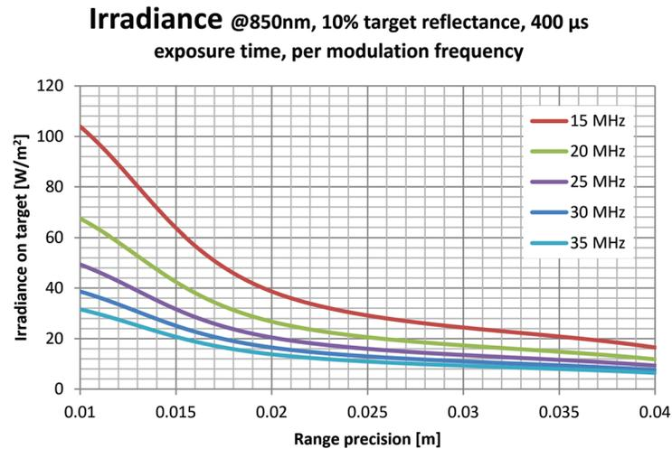
Figure 4. Irradiance on target required to reach a certain precision for different modulation frequencies lengths.
