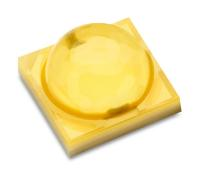
LUXEON V2 is a Chip Scale Package (CSP) based high power domed LED optimized for directional applications to continue Lumileds leadership in this category. LUXEON V2 delivers high efficacy and robustness in a 3535 package with 3-stripe footprint designed to accelerate time to market by matching the radiation pattern of LUXEON TX while improving system costs through unparalleled performance (flux and efficacy).
