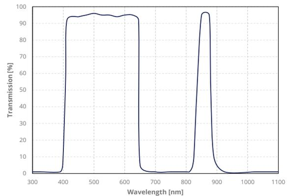
b). Dual Band pass filter visible +850nm
