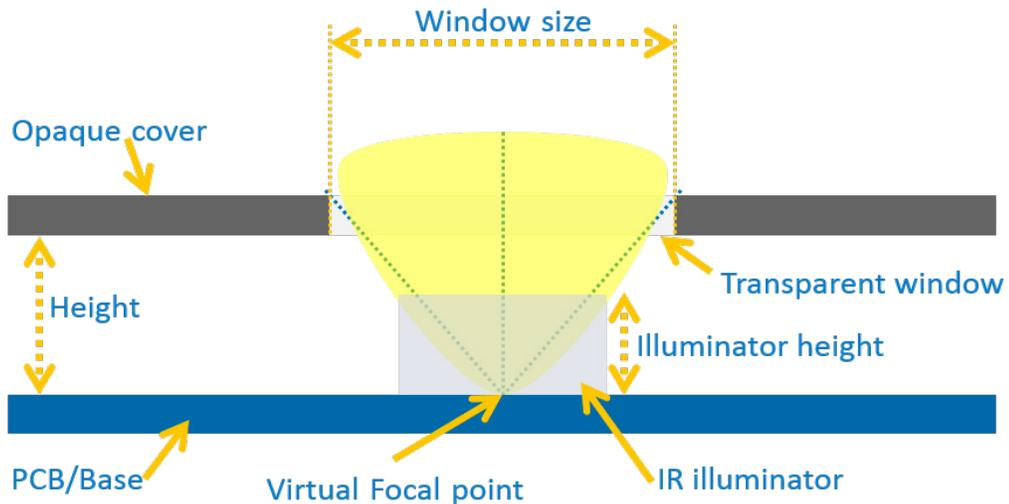
Figure 12. Schematic of IR illuminator within the facial recognition module.
