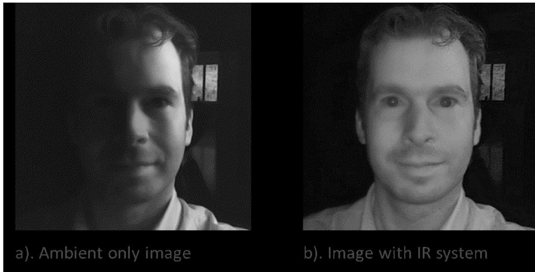
Figures 3a and 3b. Example of the advantage NIR illumination.
