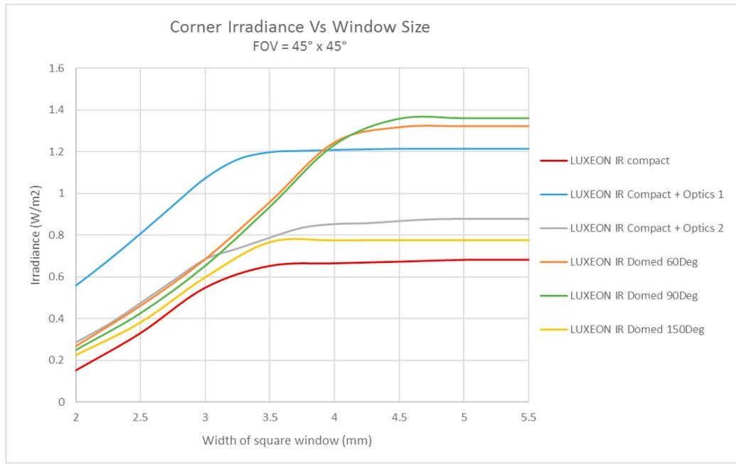
Figure 13. Impact of window size on corner irradiance with window height of 3mm.
