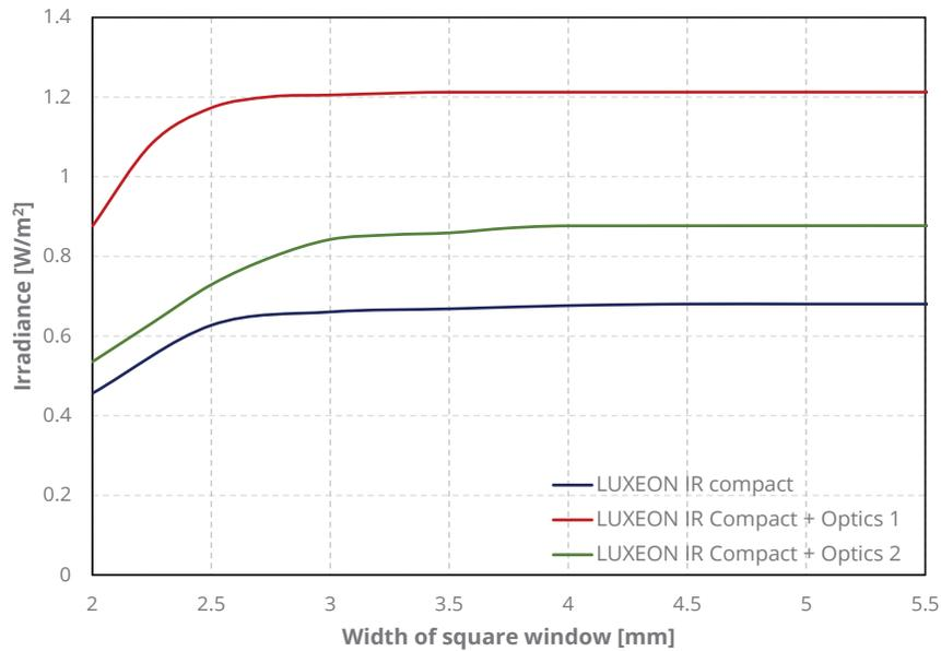
Figure 14. Impact of window size on corner irradiance with window height of 2mm.
