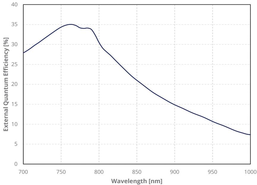
Figure 8. Example of a spectral sensitivity curve for a Si based camera sensor.
