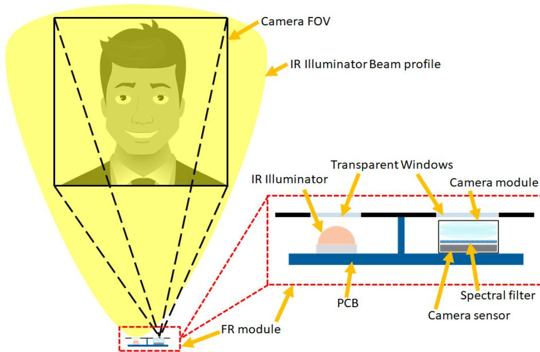
Figure 2. Schematic of the facial recognition module and hardware.
