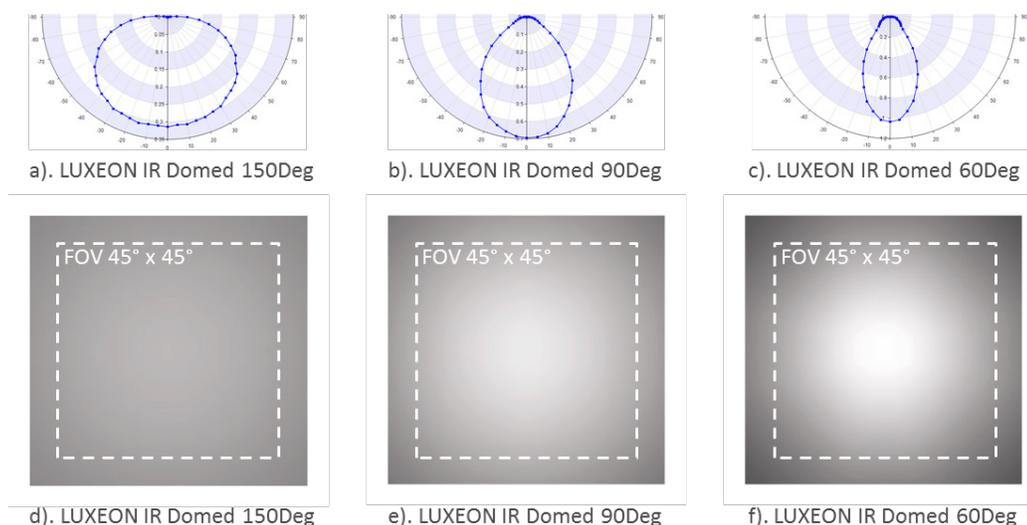
Figure 10. Radiation profiles and their performance on target (window height = 3mm).
