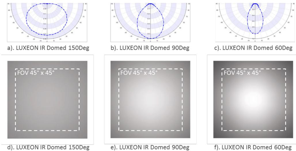
Figure 11. Radiation profiles and their performance on target (window height = 2mm).
