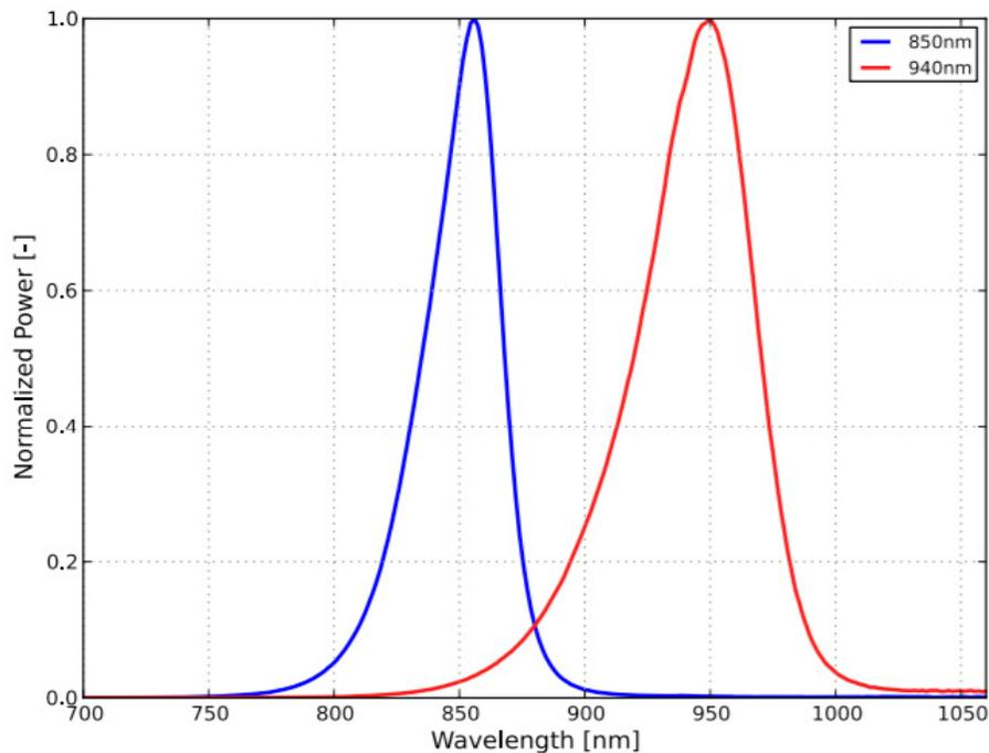
Figure 4. Spectral Power Distribution (SPD) of the LUXEON IR products.
