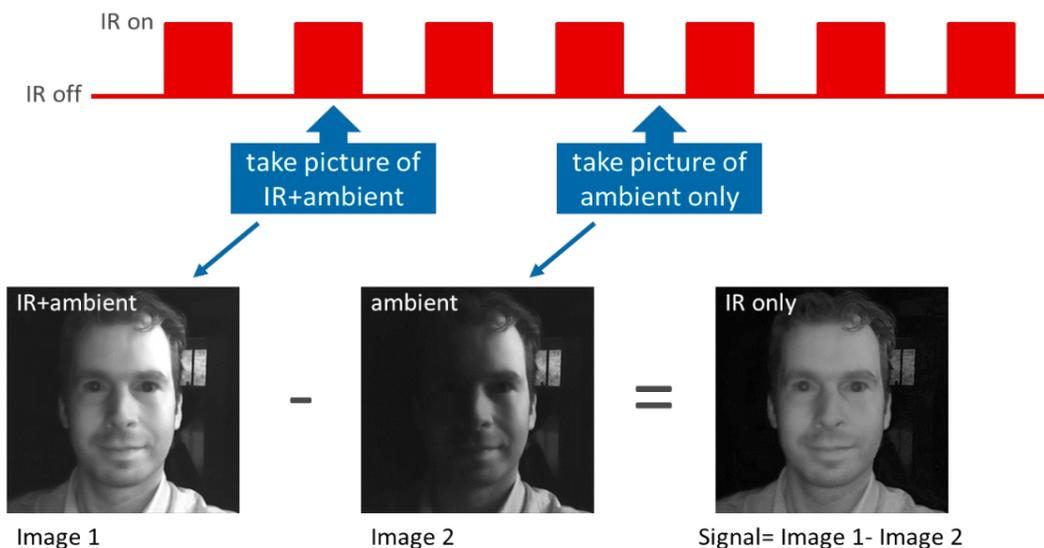
Figure 6. Example of reducing the ambient light impact.
