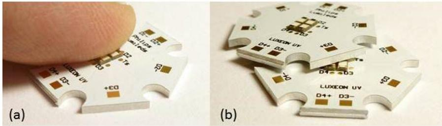
Figure 4. Do not touch the top of surface of the LUXEON UV U Line emitter when handling a finished board (a) or stack boards with one or more LUXEON UV U Line emitters on top of each other (b).
