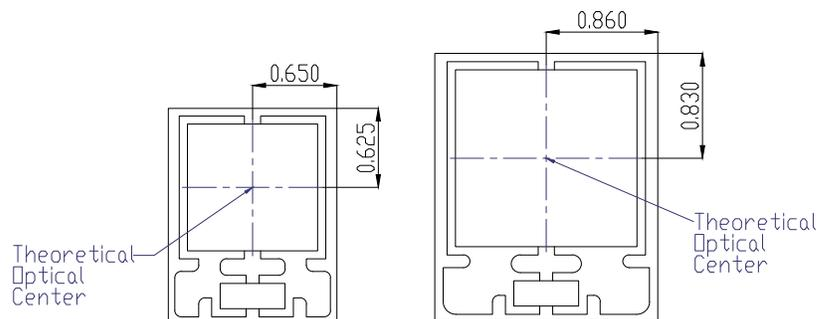
Figure 2. The optical centers of the LUXEON UV U Line emitter (in mm).
