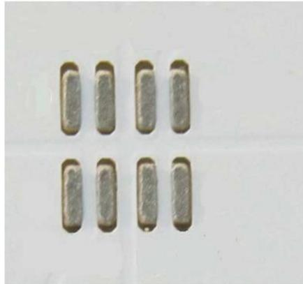
Figure 6. An example of good stencil printing on 4-up MCPCB star board.
