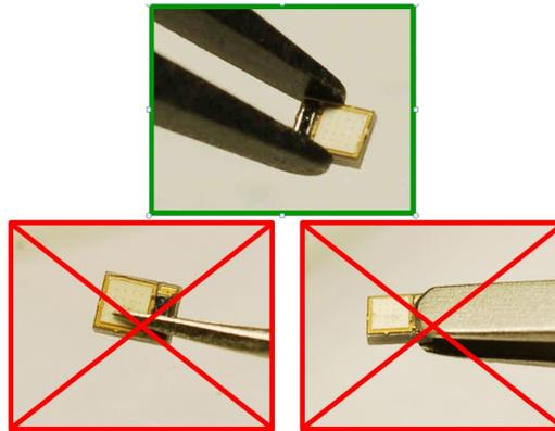
Figure 3. Correct handling (top) and incorrect handling (bottom) of LUXEON UV U Line emitters.
