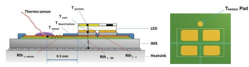
Figure 12. Temperature probing by thermo sensor (schematically).
