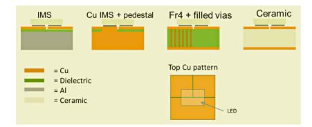
Figure 10. Layer stacks and top side pattern.
