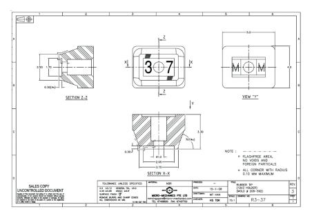
Figure 16. Standard nozzle for LUXEON Altilon SMD 1x5 and 1x4 LED array.
