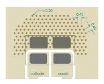
Figure 11. FR4 design with filled and capped via.
