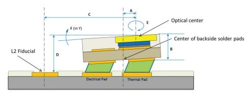
Figure 18. L1 and L2 tolerance definition.
