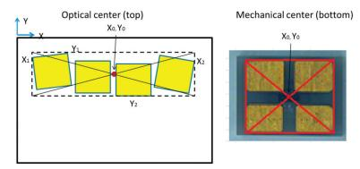
Figure 19. Definition of optical and mechanical center for LUXEON Altilon SMD.
