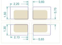
D: 1x4, 8 mil thick stencil with 150% aperture plus 100 µm offset —> 185 µm bond line thickness
