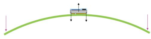
Figure 22. Forces acting onto package when board is bent.
