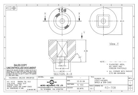
Figure 17. Standard nozzle for LUXEON Altilon SMD 1x3 and 1x2 LED array.
