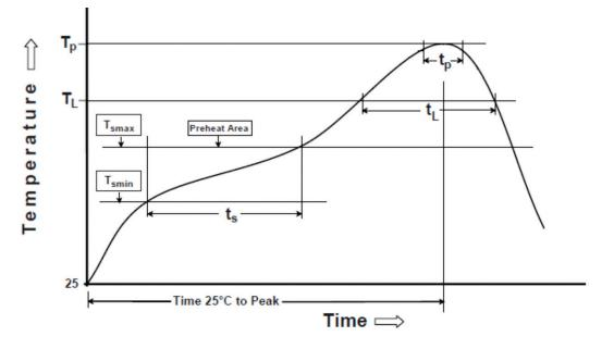
Figure 14. Reflow profile LUXEON Altilon SMD using SAC solder paste.
