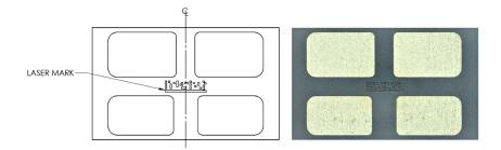
Figure 4. Example of a dot matrix code on bottom side of LUXEON Altilon SMD.
