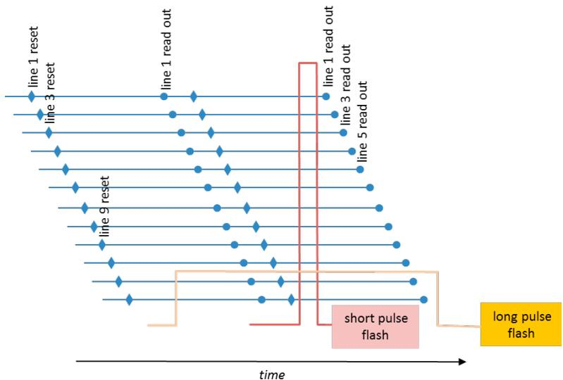
Figure 5. Rolling shutter time sequence with integration times and readout.
