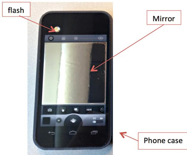
Figure 6. Camera flash for selfie demonstrator.
