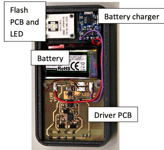
Figure 7. camera flash for selfie demonstrator (inside).
