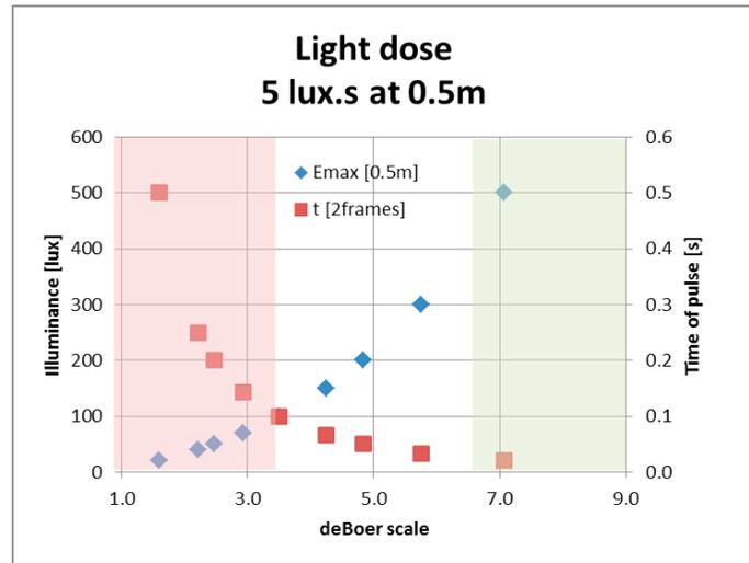
**Figure 4. Illuminance and pulse length for constant light dose vs. deBoer scale.**
