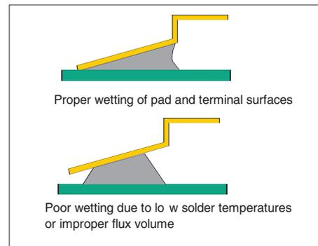
Figure 11. Solder Joint Inspection.
