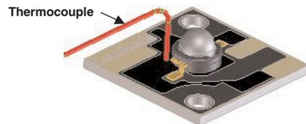
Figure 10. Location of thermocouple to monitor  $T_{Board}$ .
