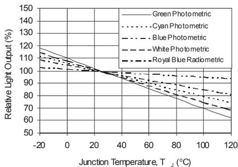
**Figure 17. Temporary InGaN Light Output Loss (typical performance).**
