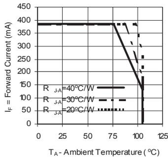
**Figure 33. Maximum Forward Current vs. Ambient Temperature.**
