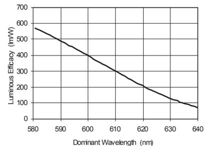
**Figure 6. Luminous Efficacy vs. Dominant Wavelength for AlInGaP Material.**
