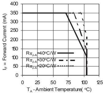
**Figure 34. Maximum Forward Current vs. Ambient Temperature.**
