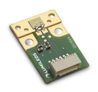
LUXEON Altilon H1K PnP is a fully integrated solution optimized for headlight applications, meeting both SAE and ECE color specifications. This solution minimizes time to market and simplifies supply chain by reducing optical and mechanical design efforts with electrical connectors. Combined with LUXEON Altilon LEDs, LUXEON Altilon H1K PnP provides the same powerful performance guaranteed by LUXEON LEDs.
