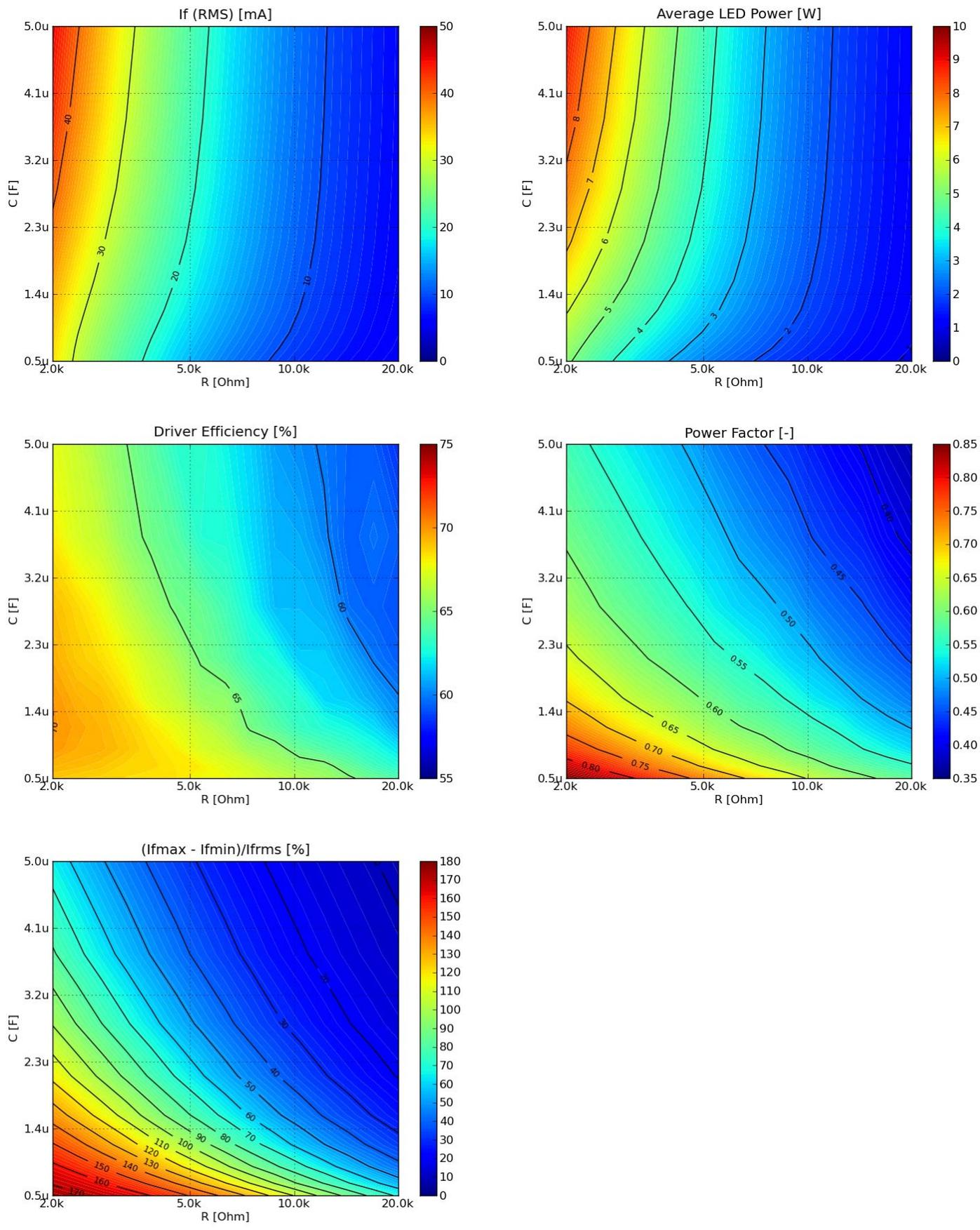
**Figure 13. Simulated performance metrics for LUXEON H 200V in Driver Circuit B as function of  $R_{out}$  and  $C_{out}$  ( $V_{ac} = 230V, 50Hz$ ).**
