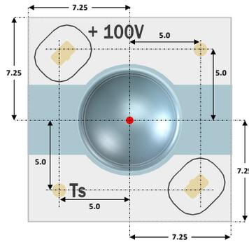
**Figure 2. Fiducial marks on the top of the LUXEON H emitter provide the most accurate method to locate the theoretical optical center. The two corner cut-outs near the fiducials are designated for M3 screws to secure the LUXEON H emitter onto a heat sink. All dimensions in mm.**
