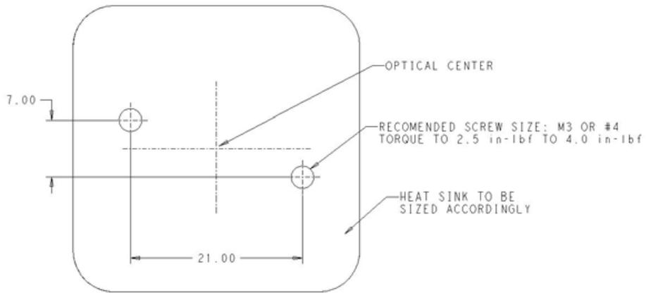
**Figure 6. Reference layout and dimensions of the holes that need to be drilled into the heat sink to align and secure the LUXEON H emitter with the TE Connectivity LED Holder, Type LH. All dimensions are in mm.**
